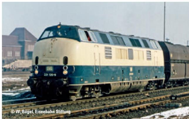
**Prototype:** German Federal Railroad (DB) class 221 (former V 200.1) heavy diesel hydraulic general-purpose locomotive. The locomotive looks as it did in Era IV around 1985.
